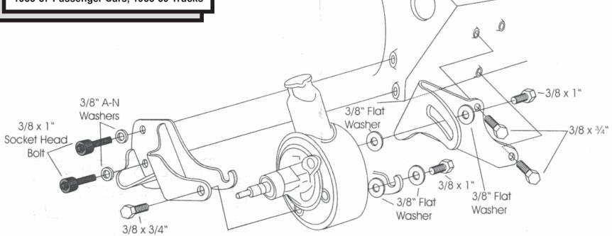
NOTE: If your pump has a stud at the lower rear pivot point, it must be removed and the 1" bolt and 3/8" flat washers used...
